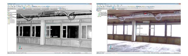
The individual scans of a project can be automatically combined in the SCENE software. The recorded scenery can be viewed in three dimensions in SCENE and measurements can be taken with simple tools directly in the scan data. All the scans are also available in colour and as high-contrast intensity images. In SCENE it is also possible to remove any irrelevant scan information and reduce the data volume.
