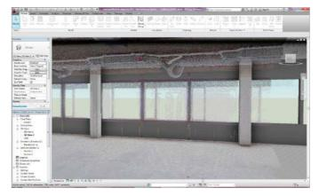
After the scan data has been prepared in SCENE, it can be transferred with no difficulty to a large number of commonly available CAD systems (such as Autodesk Revit, AutoCAD Architecture and Bentley MicroStation). There the scan data can be immediately used to produce plans of existing buildings or for the planning of conversions and extensions.  $\Sigma$
